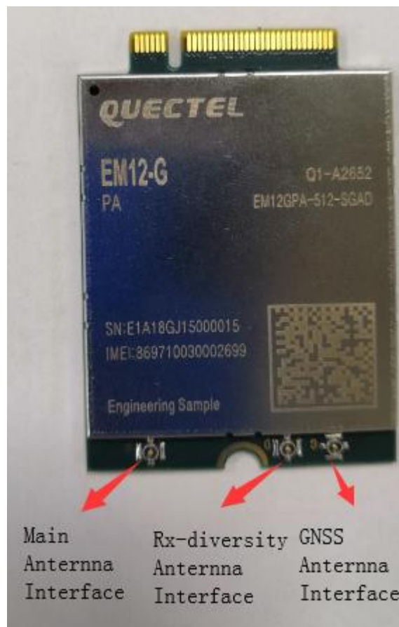
Figure 23: Antenna Interfaces on the Module
