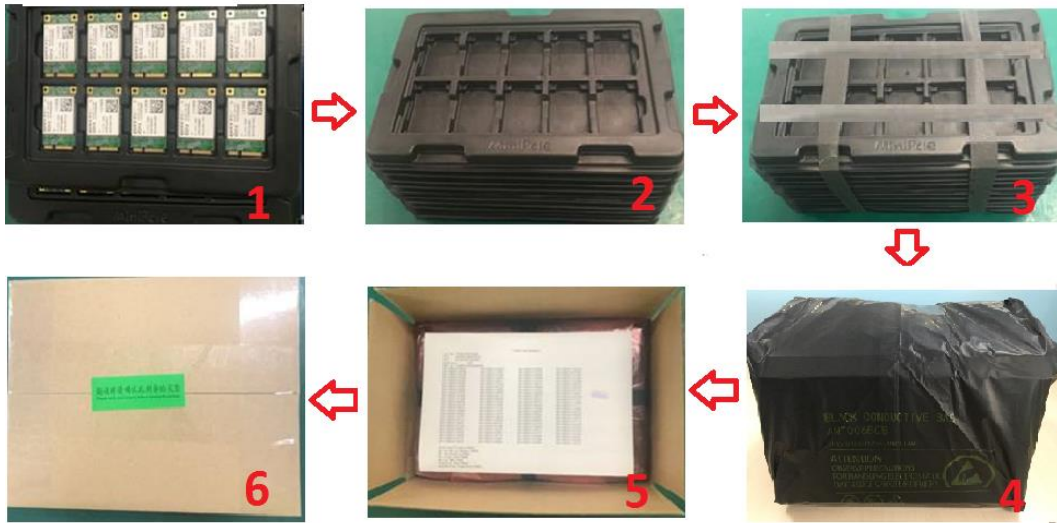
Figure 34: Tray Packaging Procedure
